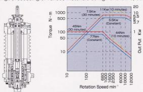
Main Spindle Motor Output: 11kW/7.5kW/5.5kW (10min./30min/Constant)
