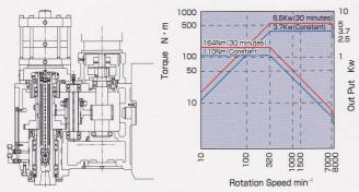
Main Spindle Motor Output: 5.5 kW/3.7 kW (30min/Constant)
